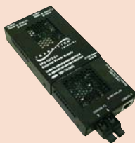
Piggy-Back Power Supply Attached to Converter
